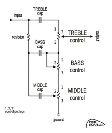
I've dispensed with off-putting things like component values that, as players rather than builders, we don't need to worry about, but the layout is complete, the real deal. It is called a stack because in an electrical diagram the sections sit on top of each other like this, incoming signal at the top, ground at the bottom.
